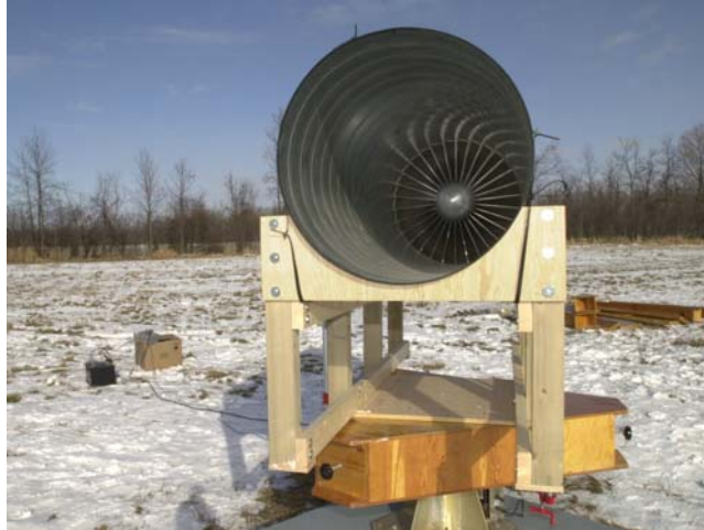
Fig. 5 Test cylinder with skewed blade assembly
