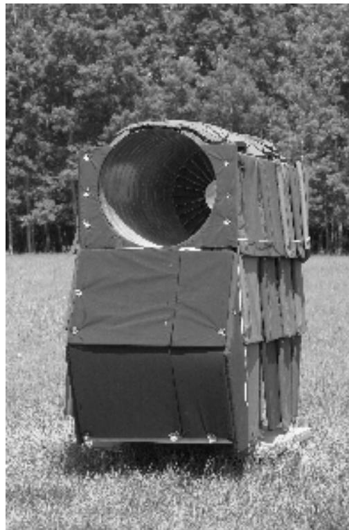
Figure 2 A picture of the full-size engine-duct mock-up with RAM tiles covering the exterior of the experimental set-up.
