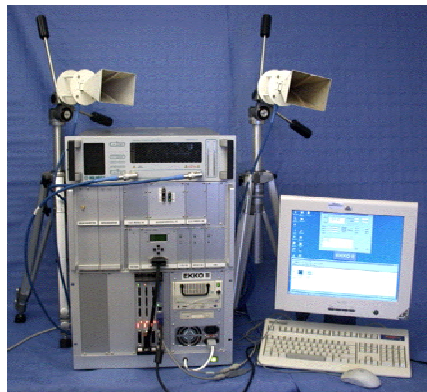
Figure 1: EKKO II in X-band configuration
